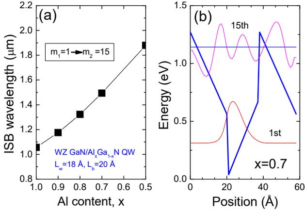
Fig. 1. (a) Intersubband transition wavelength as a function of Al content in the barrier for the absorption from the first subband ( $m_1=1$ ) to the 15th higher subbands ( $m_2 = 15$ ) of (0001)-oriented wurtzite GaN/Al<sub>x</sub>Ga<sub>1-x</sub>N QW structure with  $L_w = 18 \text{ \AA}$  and  $L_b = 20 \text{ \AA}$  and (b) potential profile and the wave functions for 1st and 15th subbands at zone center for the QW structure with  $x=0.7$ .
