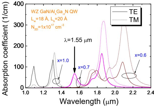
Fig. 2. TE(solid line)- and TM(dashed line)-polarized absorption spectra of (0001)-oriented wurtzite GaN/Al<sub>x</sub>Ga<sub>1-x</sub>N QW structure ( $L_w = 18 \text{ \AA}$ ,  $L_b = 20 \text{ \AA}$ ) with several Al contents in the barrier.
