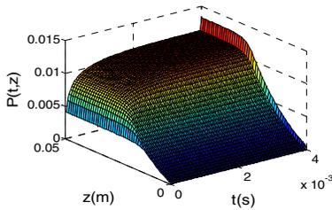
Fig. 1: Example illustrating that, for a constant pump power, the ASE power for each  $z$  reaches a stationary value after a transient time. In this example, the signal is launched at  $t = 4$  ms. The optimum fiber length corresponds to the  $z$  from which no further power increase is achieved by increasing  $z$ .
