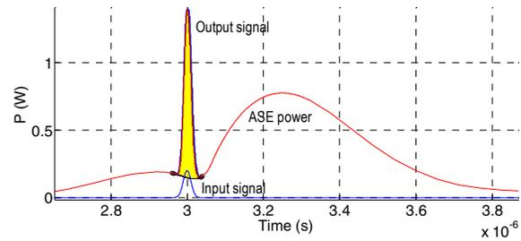
Fig. 3: Calculation of the signal energy for a pulsed pump power, which should be broader than the signal pulse and synchronized with it.
