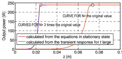
Fig. 2: Example illustrating that, for a constant pump power and without input signal, the curve of the evolution of the ASE power with  $z$ , for any  $t$  that is large enough, reaches a stationary shape that coincides with that obtained by solving the simplified equations in stationary state. In the case of low attenuation of the host material, the optimum fiber length is inversely proportional to the dopant concentration  $N$ .
