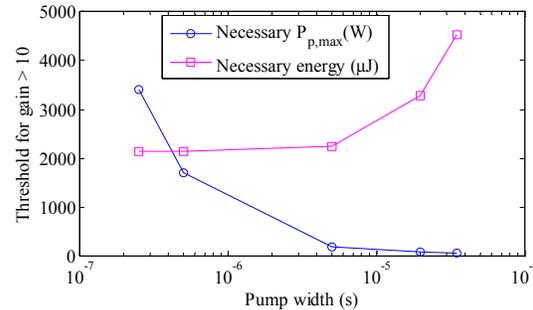
Fig. 4: Example illustrating that a constant gain (e.g. 10) corresponds to constant pump energies for small pump widths, whereas this constant gain corresponds to constant peak powers for sufficiently large pump widths.
