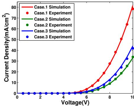
Fig. 3: The current-voltage curve of experiment and simulation. Red line means result of case.1, blue line means result of case.2 and green line means result of case.3. The dot is experiment data, the solid line is simulation result.
