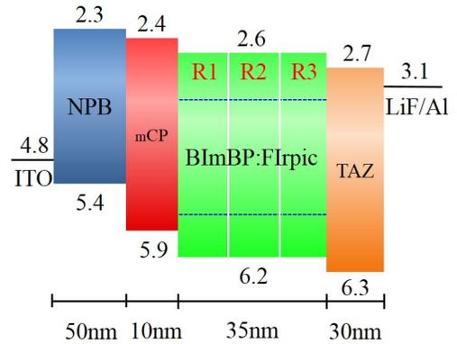
Fig. 1: Structure of OLEDs, where NPB is the hole injection layer (HIL), mCP is the hole transport layer, BImBP:Firpic is the emitting layer (EML) and TAZ is the electron transport layer (ETL).
