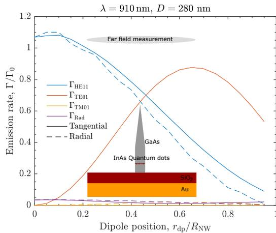
Fig. 2. The normalised spontaneous emission rate for a dipole with a wavelength of 910 nm located in a tapered nanowire with a diameter of 280 nm as illustrated in the sketch.
