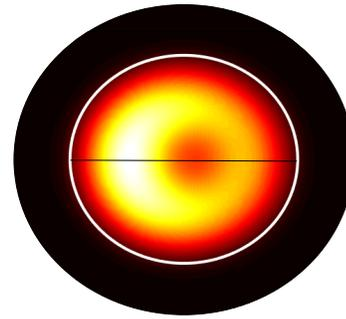
Fig. 3. Far-field pattern of the TE01 and HE11 mode in a nanowire, where the dipole is located at a radial offset of  $0.6 R_{\text{NW}}$  to the right of the centre of the mirror symmetry line.
