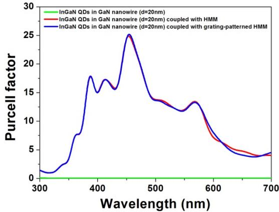
Fig. 2. Purcell factor as a function of wavelength for the InGaN/GaN NQDs, InGaN/GaN NQDs coupled with HMM and InGaN/GaN NQDs SPS coupled with grating-patterned HMM.
