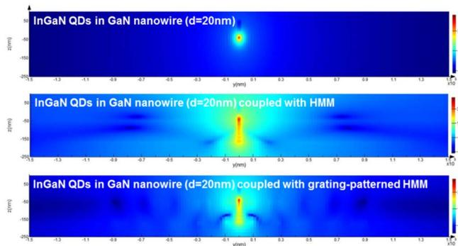
Fig. 3. The electric field emitted by a horizontal dipole embedded in the GaN nanowire, GaN nanowire coupled with HMM and GaN nanowire coupled with grating-patterned HMM.
