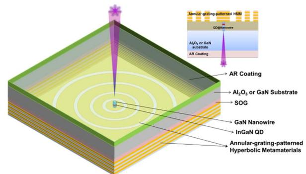
Fig. 1. Schematic of the InGaN/GaN NQDs SPS coupled with grating-patterned HMM.
