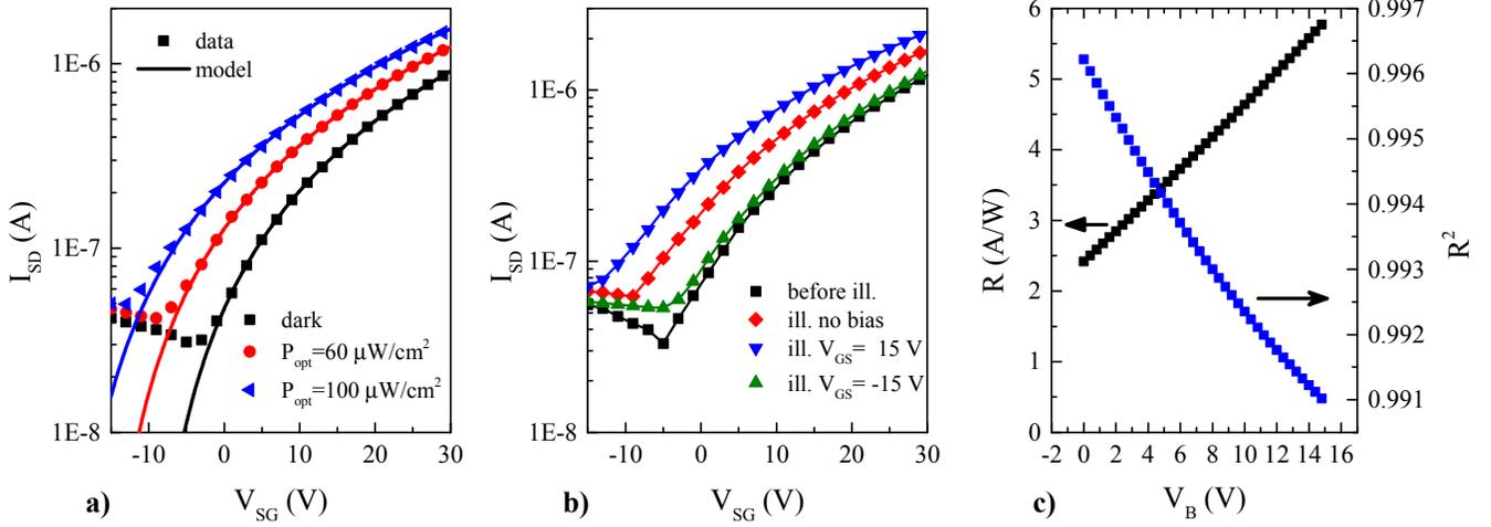
Fig. 1. a) Transcharacteristics of pentacene-based OPTs ( $V_{SD}=15$  V) in dark and under light at 550 nm with different optical power densities; experimental data are fitted with (1) and (2); b) transfer curves collected in dark before and after illumination; the devices were irradiated for 5 min without bias or under stress conditions with positive or negative gate bias; c) extracted responsivity and the coefficient of determination correlating photocurrent and optical power.
