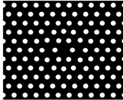
Fig. 3. Optimized Hz-polarized PhCC using shape optimization for given frequency  $\omega_0 = 0.2249 * 2\pi/a$ .
