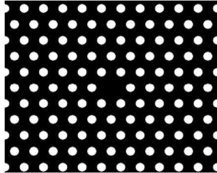
Fig. 1. Illustration of PhCC with triangular patterned air holes.
