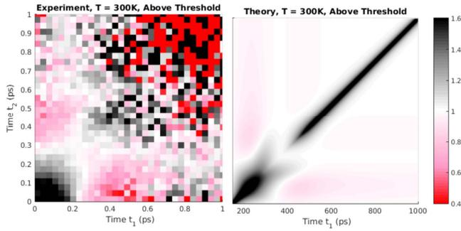
**Figure 2** Two-time map of the second-order photon correlation function  $g^{(2)}(t_1, t_2)$  for a nanolaser under pulsed excitation. The diagonal corresponds to  $\tau=0$ . Left: Measurement on a high-Q photonic-crystal nanolaser at room temperature. Right: Microscopic laser theory.
