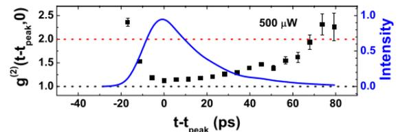
**Figure 1** Time-resolved emission intensity (solid) and second-order photon correlation function  $g^{(2)}(t, \tau=0)$  (dots) as measured on a quantum-dot micropillar laser. Adapted from [2].
