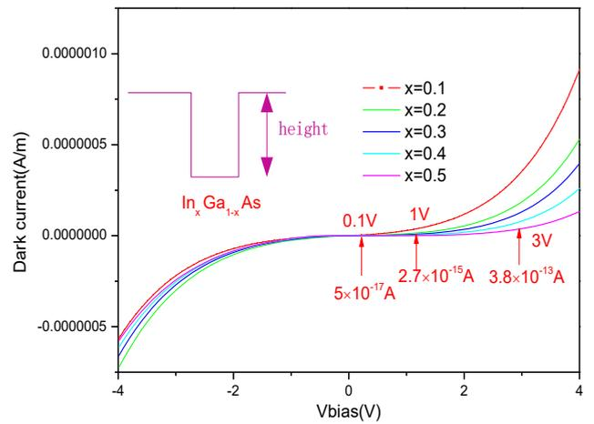
Fig.2. The different dark current at the width quantum well
