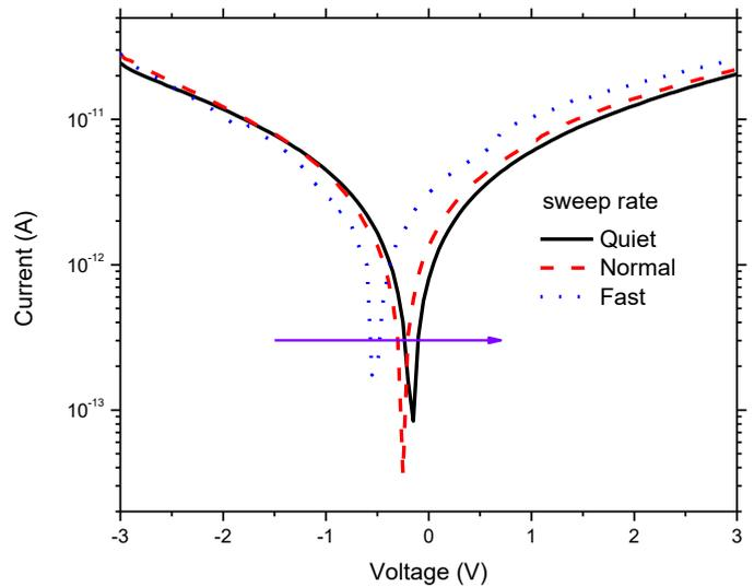
Fig.3 dark current test with three scan rate—quiet, normal, fast
