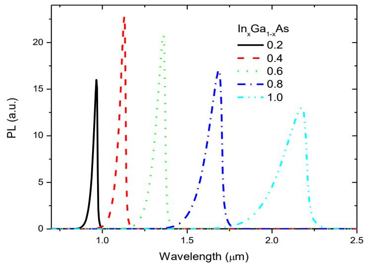
Fig.4. Photoluminescence spectra simulated under different the component of the In. (x=0.2, 0.4, 0.6, 0.8, 1)
