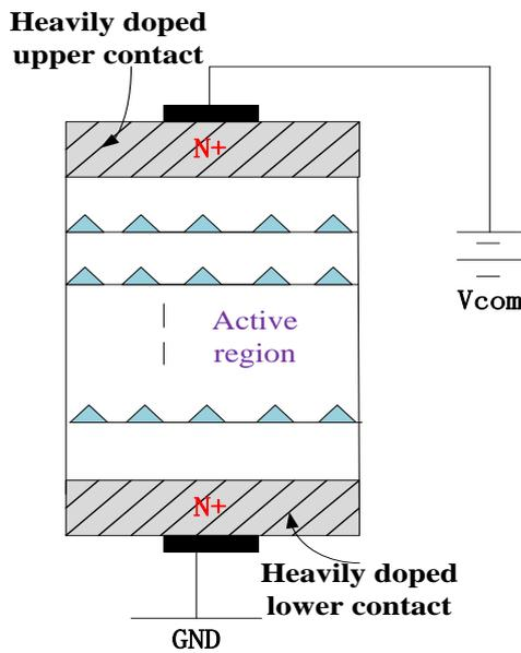
Fig. 1 The schematic structure of self-assembled QDIPs showing the active regions and the top and bottom contacts.
