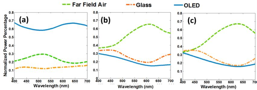
Fig. 2 (a) Far-field power for a conventional OLED structure, (b) structure modified organic layer on the emissive layer and (c) OLED structure with optimized ITO.
