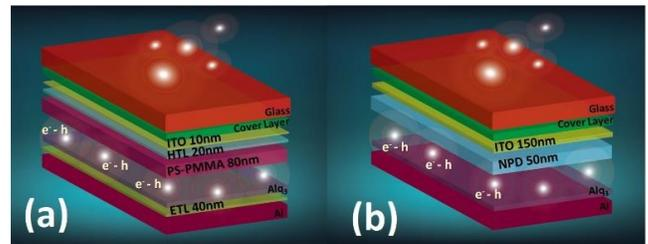
Fig. 1 (a) A conventional OLED structure and (b) modified organic layer on emissive layer and optimized ITO structure.
