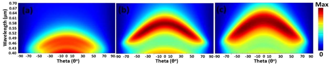
Fig. 3 (a) Intensity profiles for conventional OLED structure, (b) structure modified organic layer on the emissive layer and (c) OLED structure with optimized ITO.
