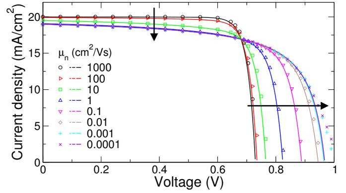
Fig. 2. Current voltage characteristics under illumination for different mobilities. The parameters are:  $N_c = 10^{19} \text{ cm}^{-3}$ ,  $E_g = 1.42 \text{ eV}$ ,  $\phi_b = 0.2 \text{ eV}$ ,  $v_s = 10^6 \text{ cm/s}$ ,  $qGL = 20 \text{ mA}$ ,  $L = 100 \text{ nm}$ . The symbols give the results of numerical drift-diffusion simulations.
