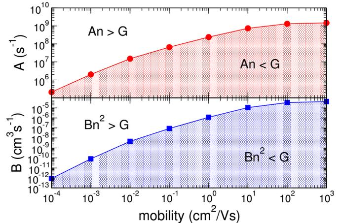
Fig. 3. Recombination parameters required such that Shockley-Read-Hall or direct/bimolecular bulk recombination becomes dominant.
