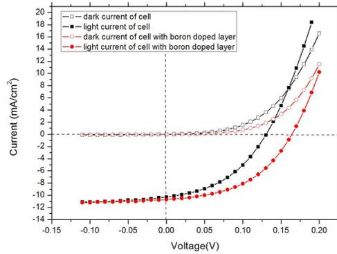
Fig.4 IV characteristics of the device under AM1.5 illumination
