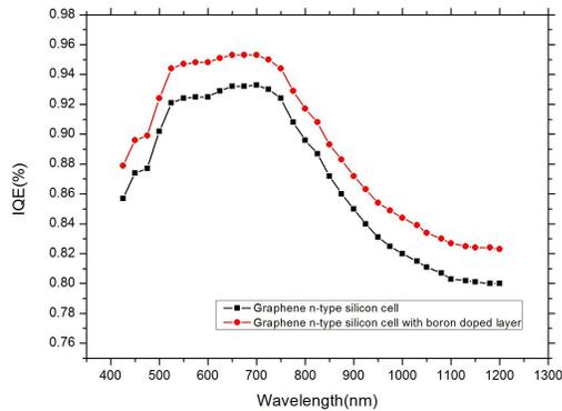
Fig.3 IQE of the device under AM1.5 illumination
