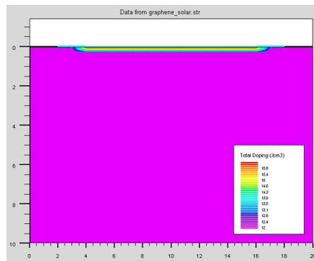
Fig.1 Cross section of the graphene silicon junction solar cell with inverse doped surface layer
