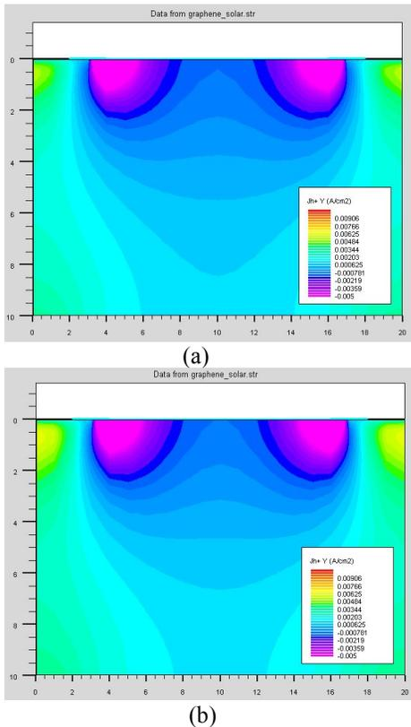
Fig.2 Hole current density distribution at Y direction of the device: (a) graphene n-type silicon solar cell (b) graphene n-type silicon solar cell with boron doped layer
