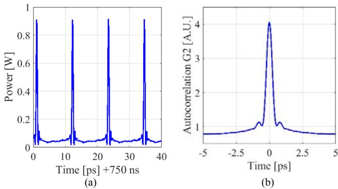
Fig. 2 Calculated pulses after GDD compensation (a) and corresponding autocorrelation (b).
