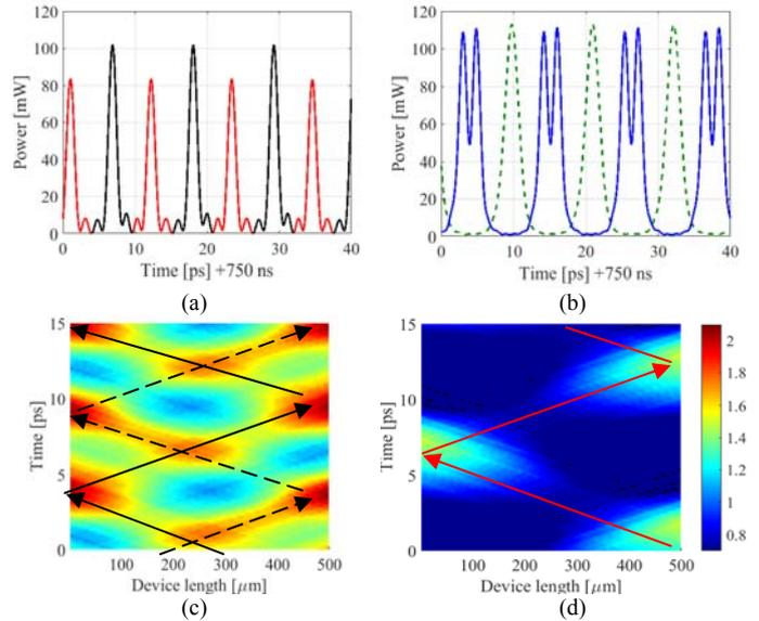
Fig. 3 Pulse train due to the central modes of the optical spectrum (a); pulse train due to the lateral modes on the blue (blue line) and red (dashed line) wavelength side of the optical spectrum. Photon density resonant with the GS of the central (c) and lateral (d) QD sub-groups.
