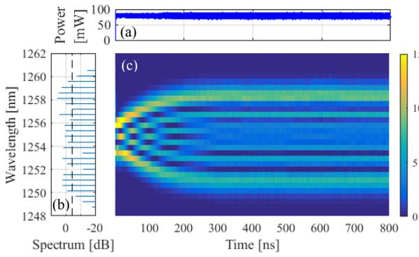
Fig. 1 (a) Power versus time, (b) optical spectrum, (c) mode intensity versus time.
