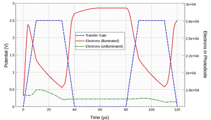
Fig. 4. Transient characteristics showing the applied transfer gate voltage (dash line), electrons generated under illuminated (solid line) and unilluminated (dash-dot line) conditions.
