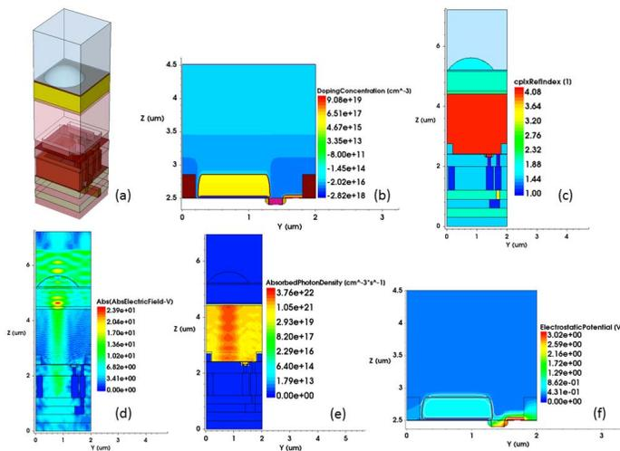
Fig. 3. Complete simulation flow for CIS modeling: (a) BSI CIS structure (b) Net doping concentration from Process simulation (c) Refractive Index profile (d) electric field,  $|E|$  (e) Absorbed photon density from FDTD (f) Electrostatic potential from electrical simulation. Note that cross-sections shown in b through f are taken at  $x=1.2\mu\text{m}$  (middle of lens).
