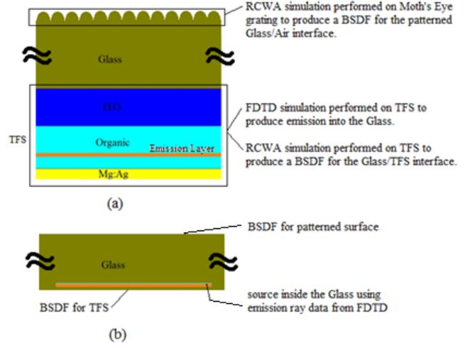
Fig. 1. (a) OLED structure showing where the EM (FDTD, RCWA) methods were applied to generate data for ray-tracing model. (b) Simplified OLED structure used for ray-tracing simulation where the EM results were used.
