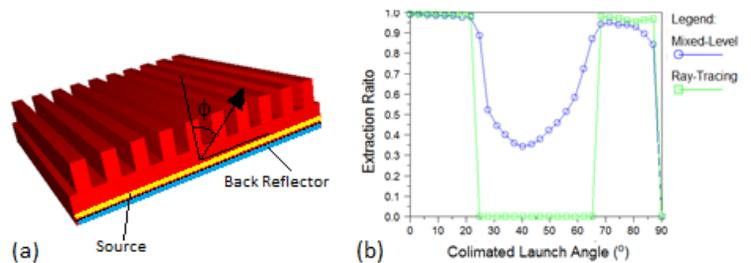
Fig. 2. (a) 1D rectangular surface grating with back reflector. The duty cycle for the rectangular grating was 0.5,  $\phi$  is the collimated launch angle. (b) Light extraction ratio into air, with  $\text{Period}/\lambda \sim 71$ , calculated via the two simulation methods mixed-level (solid with circles) and ray-tracing (dashed with squares)
