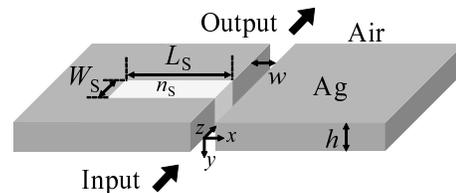
Fig. 1. Stub-type filter.
