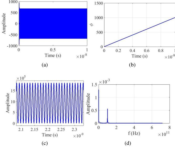
Fig. 2: (a) Electric field distribution, (b) instantaneous phase, (c) time domain beat signal, (d) frequency domain beat signal for no lock-in case i.e.  $\Omega_r \gg \Omega_L$
