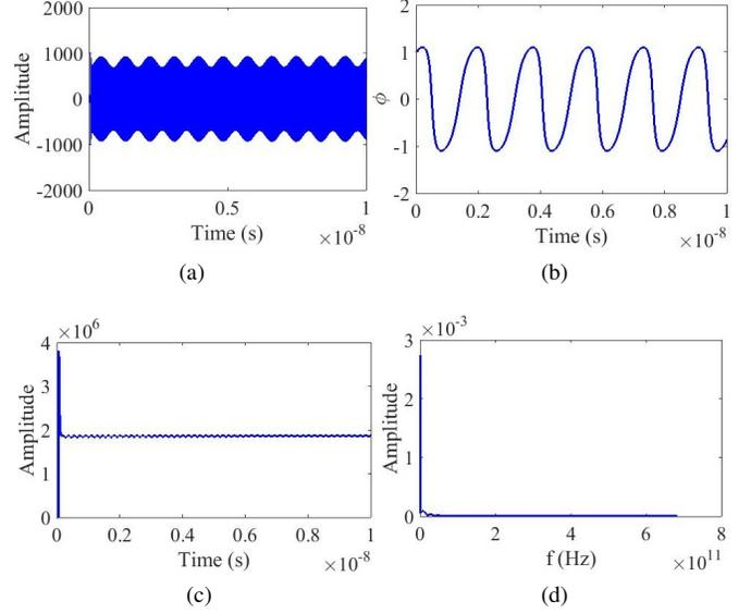
Fig. 3: (a) Electric field distribution, (b) instantaneous phase, (c) time domain beat signal, (d) frequency domain beat signal for lock-in case i.e.  $\Omega_r < \Omega_L$
