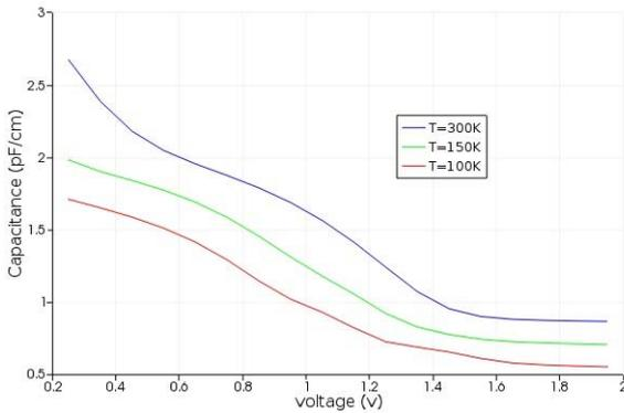
Fig. 5. C-V measurements performed at T = 300 K, 150 K, and 100K.
