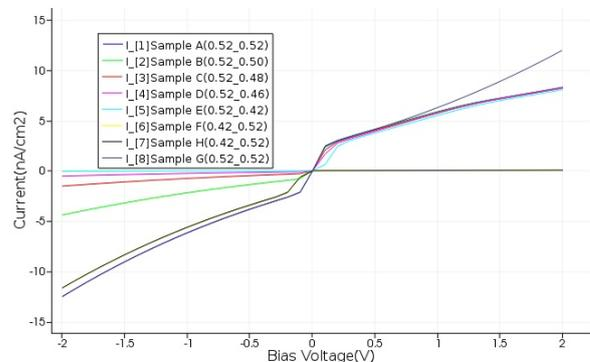
Fig. 3. I-V of all samples applied by voltage from  $-2\text{V}$  to  $2\text{V}$ .
