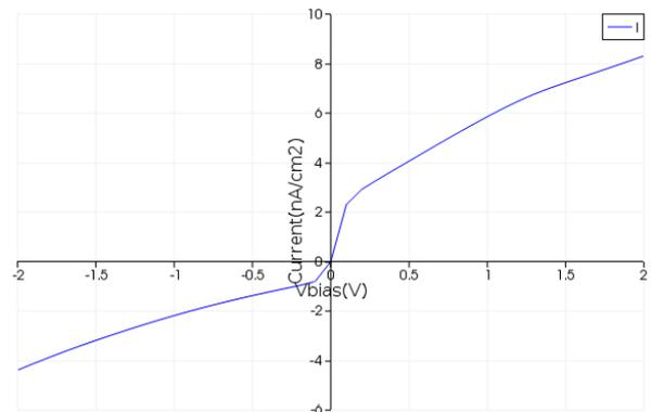
Fig. 2. I-V at different bias voltage, from  $-2\text{ V}$  to  $2\text{ V}$ .
