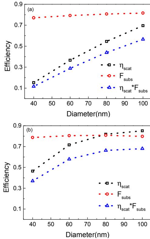
Fig.3 Average scattering and coupling efficiency calculated over the light trapping spectral region for a Si substrate (500 nm to 1200 nm) for rear located particles, varying diameter from 40 to 100 nm.
