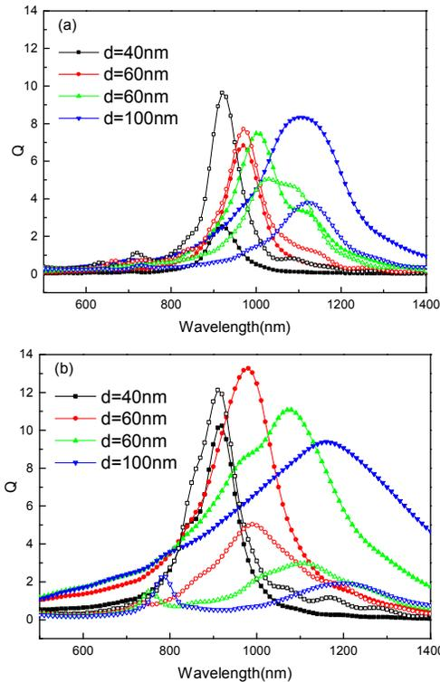
Fig.2 Calculated normalized scattering cross-section (Qscat, solid symbol line) and normalized absorption cross-section (Qabs, open symbol line) for rear located Ag nanoparticles directly on a Si substrate, Data is shown for hemispherical nanoparticles (a) extending into air and (b) extending into silicon, with diameters of 40 nm (black square), 60 nm (red circle), 80 nm (green up triangle), and 100 nm (blue down triangle)
