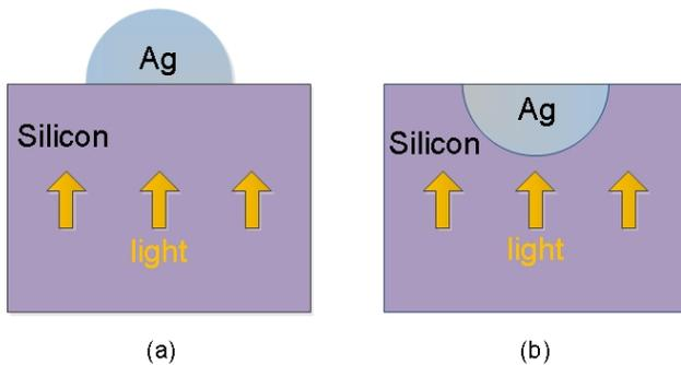
Fig.1 Schematic of the FDTD simulation model. (a) nanoparticle extending into air and (b) nanoparticle extending into silicon.
