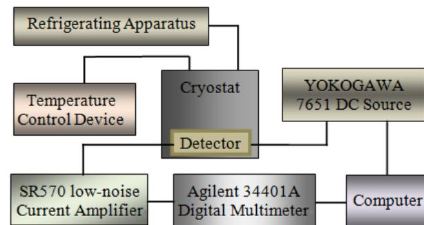
Figure1. Schematic of the experimental testing system for the measurement of dark current.
