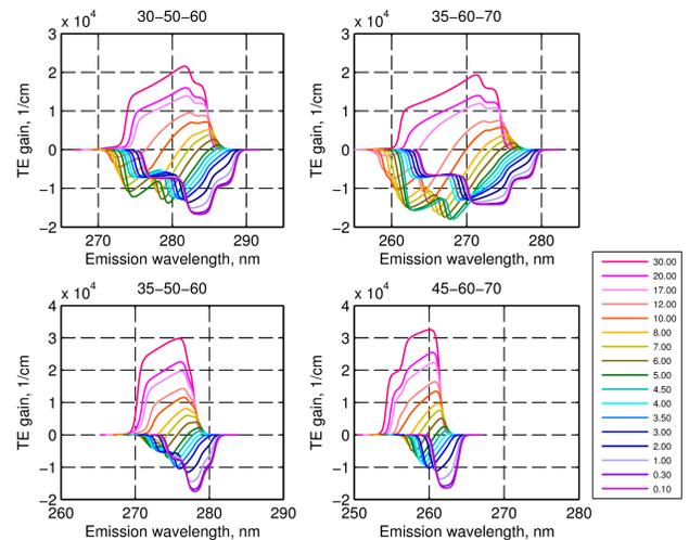
Fig. 2. TE gain spectra of selected QWs with shallow (upper subplots) and deep (lower subplots) confinement depth. The legend indicates QW carrier concentration in  $10^{12}/\text{cm}^2$ . QWs are labeled as in Fig. 1
