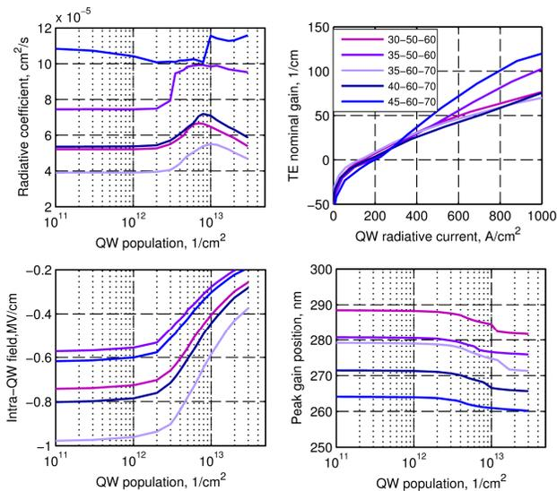
Fig. 1. Calculated characteristics of DUV-emitting QWs with different confinement depth. The legend indicates aluminum percent contents in QW, waveguide (barrier), and cladding layers.
