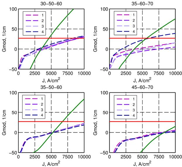
Fig. 3. Threshold condition in 4-QW DUV LD structures. Red line - total optical loss; green line - total modal gain. Dashed lines show partial modal gains of specific QWs counted from N-side of the diode. Shallow-QW LD structures (lower subplots) demonstrate more uniform MQW injection but suffer from insufficient QW populations and lower gain.
