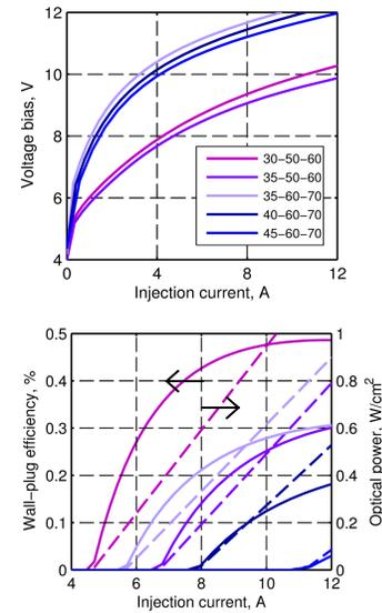
Fig. 4. Output characteristics of 4-QW LD structures specified by the legend in the upper subplot. LD performance degrades with decreasing active QW depth and/or increasing overall aluminum composition; combination of both trends being detrimental for structure 45-60-70 (structure codes: QW-Waveguide-Cladding aluminum in percent).
