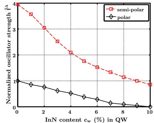
Fig. 2. Normalized oscillator strength in polar (black solid) and semi-polar (red dashed)  $\text{In}_{0.25}\text{Ga}_{0.75}\text{N}$  QDs embedded in QW as a function of the In content of the QW,  $c_w$ .
