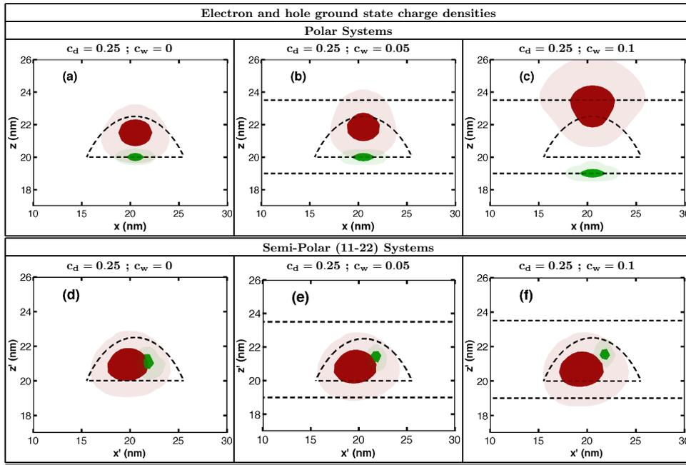
Fig. 1. Electron (red) and hole (green) ground state charge densities in polar (top) and semi-polar (bottom) DWELLS for different In contents of the well surrounding an  $\text{In}_{0.25}\text{Ga}_{0.75}\text{N}/\text{GaN}$  QD. Dashed lines indicate QD and well interfaces.
