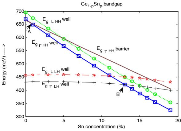
Fig. 2. Bandgap of strained GeSn as a function of Sn where,  $z$  is position variable,  $\psi$  is wave function,  $E_p$  is Eigen energy,  $m_p$  is the effective mass where suffix  $p$  stands for type
