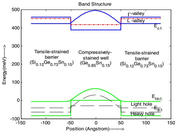
Fig. 3. Plot of energy band structure, Eigen energy and wave function in  $Ge_{0.85}Sn_{0.15}/Si_{0.12}Ge_{0.73}Sn_{0.15}$  QW of band.  $V_p$  is the potential profiles of different bands. The equation is solved using Finite Difference Method (FDM) [11]. Calculated wave functions and Eigen energies are shown
