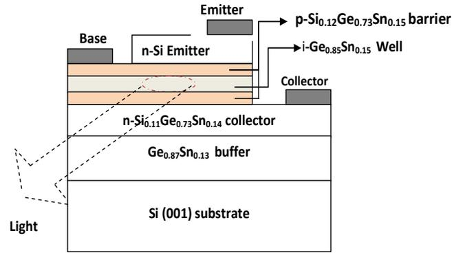
Fig. 1. Schematic structure of SiGeSn/GeSn based Transistor Laser
