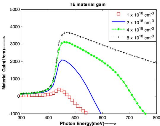
Fig. 4. TE mode gain spectra for different injected carrier densities.
