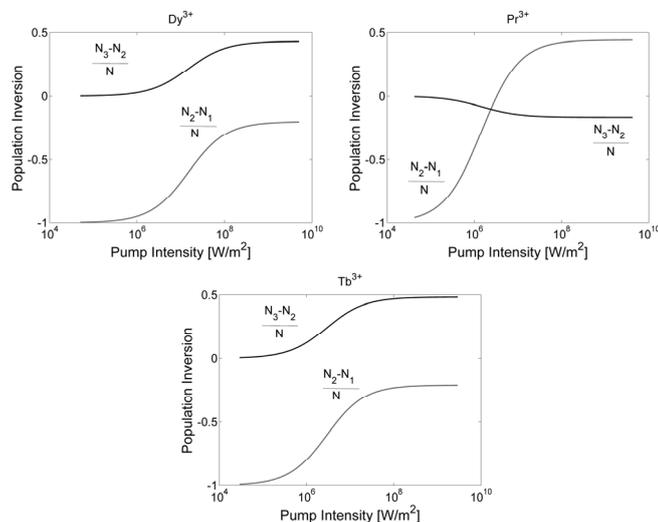
Fig. 2. Dependence of population inversion on the pump intensity for chalcogenide glass doped with trivalent dysprosium, praseodymium and terbium ions
