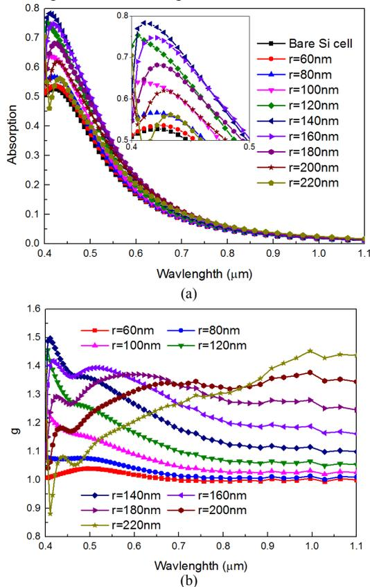
Fig.2 (a) The absorption spectra and (b) the absorption enhancement  $g(\lambda)$  of silicon in solar cells with spherical Al nanoparticles, where  $p=400$  nm
