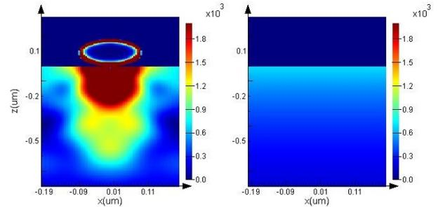
Fig.3 Visible light absorption profile of x-z cross-section at a wavelength of 500 nm in solar cells with (left) and without (right) aluminum NPs, for radius 180 nm, period 400 nm,
