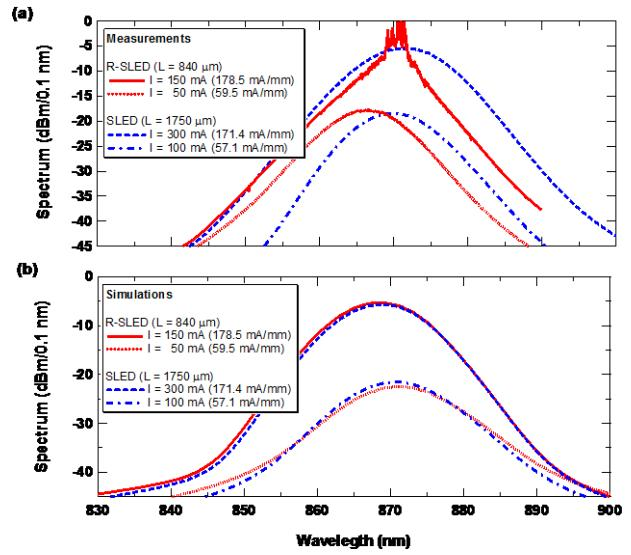
Fig. 2. (a) Measured and (b) simulated ASE output spectra of the same SLED chips as used for Fig. 1 at two different levels for the current density.
