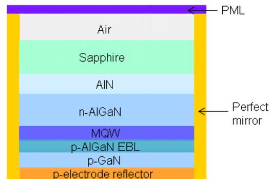
Fig. 1. Schematic side-view diagram of FDTD computational domains of flip-chip UV LED structures.
