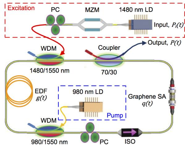
Fig. 1. Architecture of the graphene passively  $Q$ -switched excitable laser.
