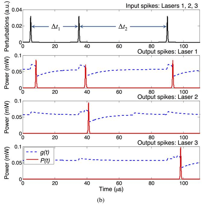
Fig. 3. (a) Schematic of a three-laser circuit to recognize specific spatio-temporal bit patterns. (b) Simulation of the spatio-temporal recognition circuit.
