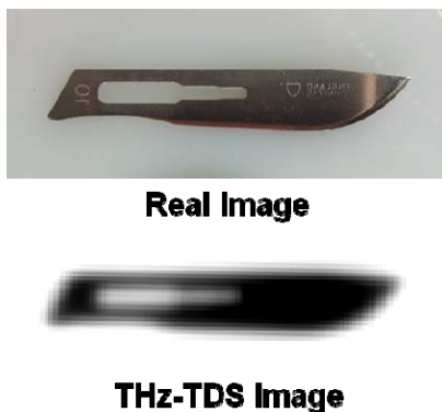
Fig. 4. Photograph of a medical knife, and its THz image measured by using the THz-TDS system.
