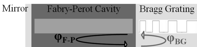
Figure 1. Schematic of a Continuum cavity, in which the round trip phase has been divided between the cavity and the Bragg Grating.
